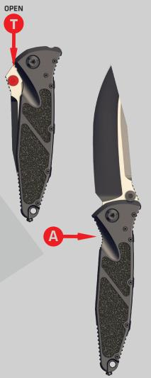
**TO CLOSE**: Press out on the lock tab and fold blade inward (A).
