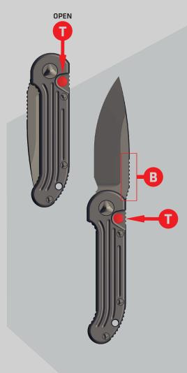
TO CLOSE: Press and hold the firing button (T) and fold blade inward with fingers safe on the spine (B). Caution: Be sure fingers are not in the path of travel!
